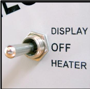
To stop the heating process, take your switch to the «**OFF**» position. The numbers on your DC will disappear.
