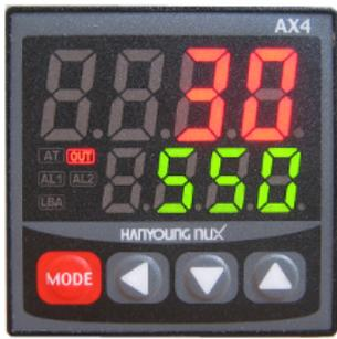
Now the upper line of your DC shows the current temperature of your heating chamber. In the lower line, it shows you the firing temperature that is set for your kiln. Now your kiln is ready. Take the switch to **HEATER** position and your kiln starts to heat.
