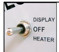
To stop the firing manually, put the 3 position switch to the **«OFF»** position. The numbers on your DC will disappear.
