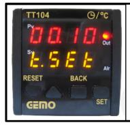
If you want to enter a firing duration (hold time), you'll need to enter min. here. Let assume we want to set a holding time of 10 min. Use **UP** and **DOWN** arrows to change the value of the upper red display to **00.10** and press **SET** key once.
