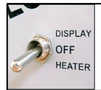
This is the 3 position switch of your kiln. When your kiln is in the **HEATER** or **DISPLAY** position, you'll see numbers on your digital controller's display. For programming take it to the **(DISPLAY)** position.
