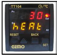
Now your kiln is ready. Take the switch to "Heater" position and your kiln starts to heat. At this position, on the upper line of your DC, you'll see the current temperature of the heating chamber and on the lower line of your DC, you'll see the target temperature and the **hEAt** word alternatively.
