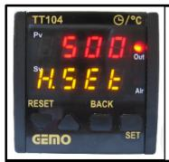
To set the target temperature press **SET** key for 2 seconds. At the lower line on you DC, you'll see **H.Set** and at the upper line you'll see a number; this is the target temperature. You can easily change it by pressing the **UP** and **DOWN** arrows.
