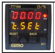
After setting your firing temperature, press **SET** key once and you'll see **t.set** which is the time that the kiln will wait at the firing temperature which you have set. If you want your kiln to fire without hold time, press **SET** key once.
