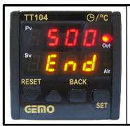
When the holding time you'll see **End** on the bottom line and your kiln will stop heating. If you didn't set a hold time, you'll see the **End** on the bottom line of your DC just after your kiln reaches to the target temperature. **End** means that the firing is over and your kiln will stop heating.
