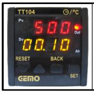
If you set a hold time, once your kiln reaches to the target temperature, on the upper line of your DC, you'll see the current temperature of the heating chamber and on the lower line of your DC, you'll see the target temperature and the hold time alternatively.
