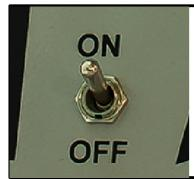
To stop the heating process, take your 2 position switch to the «**OFF**» position. The number on your DC will disappear.
