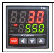
When you have entered your target temperature, just press **MODE** key for 2 seconds and your adjustment is completed. Now your kiln will start to heat.
